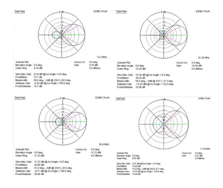
TYPEB:TwoElement40MYagi-18ftBoomA two-element 40M Yagi is a type of directional antenna designed to operate on the 40-meter amateur radio band(7.0-7.3 MHz). It consists of two elements, a driven element and a reflector element. The driven element is connectedto the transmitter or receiver, while the reflector element is placed a specific distance behind the driven element.
