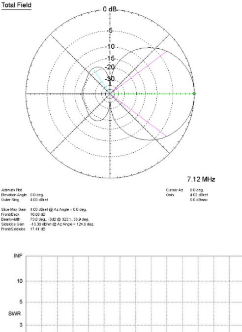
Peak Gain is shown over a dipole in Freespace Dipole in Freespace = 2.14dBi
